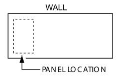
2. Secure impaling clip to wall using two screws per clip. Toggle anchors may be needed on concrete walls.
