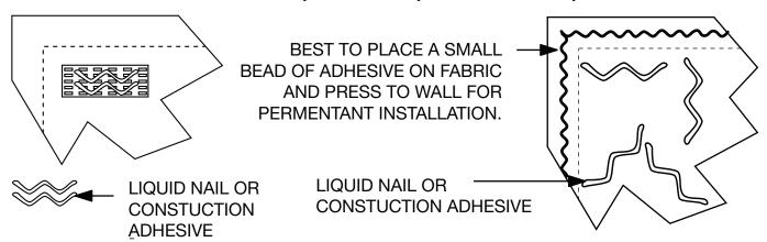
5. Press panel firmly to wall. Make sure that the fiberglass core is being impaled and not he fabric.
