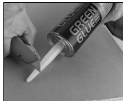
Figure 2.3: Cut a 3/8" opening in tube
