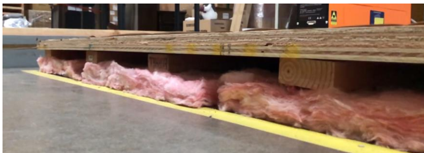
PAC-IFB2 plus sleepers 3.5" air gap 5" overall build.
