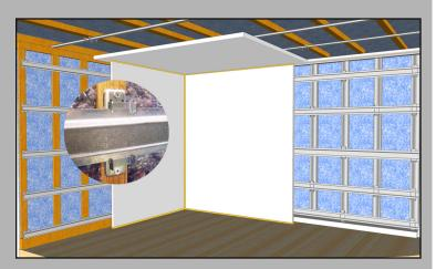
Green Glue Noiseproofing Clips install on ceilings, joists, and wall studs. Hat channel snaps into the clips, and screws are used to install the drywall directly into the channel.
