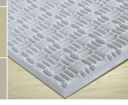
SONEX Mini Panels provide excellent sound absorption, especially in environments requiring high-frequency noise control. Made with exclusive willtec® foam, SONEX Mini Panels are a safety-minded choice for use in machine enclosures and other confined spaces. willtec foam is Class 1 fire-rated according to ASTM E 84 for flame spread and smoke density. It can withstand constant temperatures above 300° Fahrenheit, and will char, but not ignite, at temperatures above
